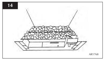
8.2 Lean the granite chippings against the burner ledges to disguise the ledges.
